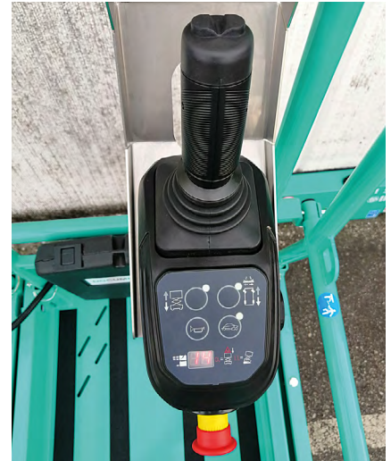
Micro Scissors come equipped with slimmed down controller
