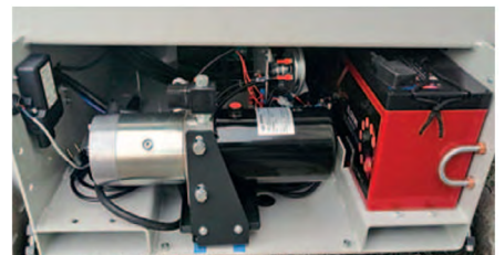
AGM batteries to ease maintenance. New disposition of hydraulic components on the lower frame which integrates forklift pockets.
